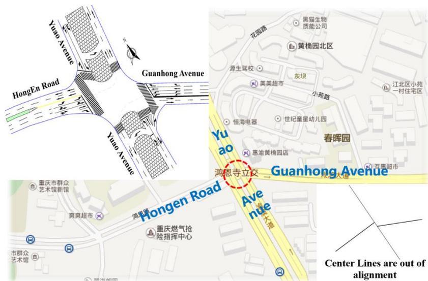
**Fig.1** Schematic diagram of the oblique dislocated intersection of Hongensi (upward vertically and down obliquely)
